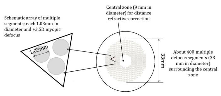
Figure 1 The design of the Defocus Incorporated Multiple Segments (DIMS) spectacle lens.
