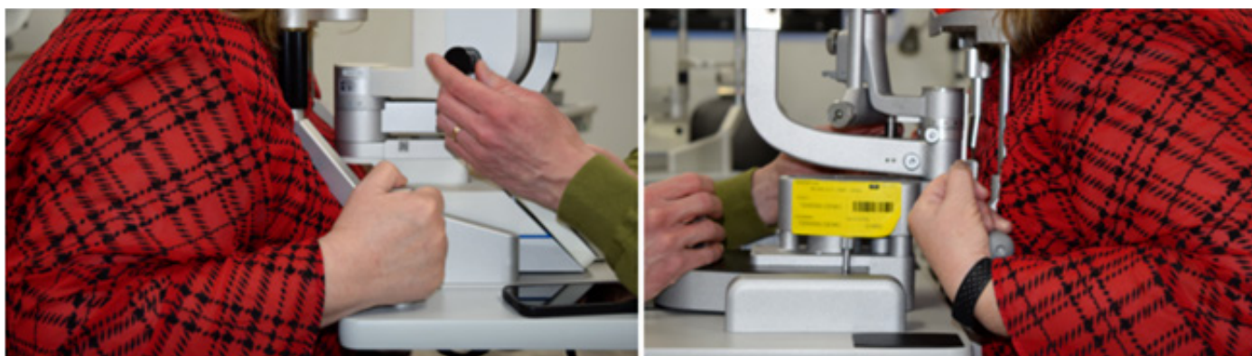
Figure 5: Direct comparison of the headrest-angle & chest-contact issue identified in certain anatomies during ergonomic evaluation
