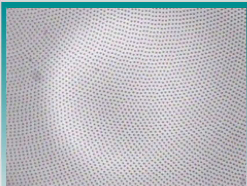
Figure 1. An example of a geometric shape created by a femtosecond laser. Multiple microscopic pulses form the desired ablation geometry.
