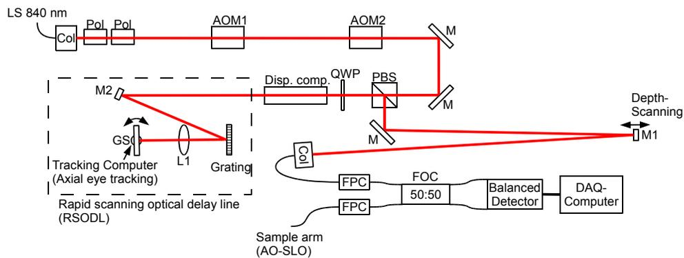
Fig. 2. Scheme of the AO-SLO/OCT reference arm. LS light source, Col collimator, Pol polarizer, AOM acousto optic modulator, M mirror, PBS polarizing beam splitter, QWP quarter wave plate, Disp. Comp. dispersion compensation, L1 lens (80 mm), GS galvanometer scanner, FPC fiber polarization controller, FOC fiber optic coupler
