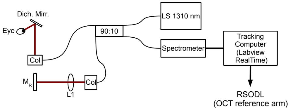
Fig. 3. Scheme of the axial eye tracking system. LS light source, Col Collimator, L1 lens, Dich. Mirr. dichroic mirror.
